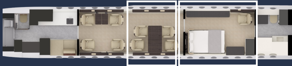
VIP Configuration Master Suite, Ultra-Wide dining area and large bathroom
